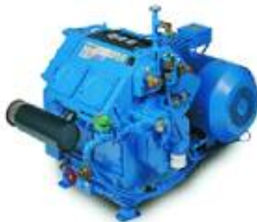
5317– 5337 Three stage, water-cooled for pressures from 580 to 1200 psig and capacities from 25 to 95 cfm.
