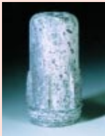
Rapid Corrosion of Untreated Aluminum
