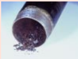
Corrosion of Piping
